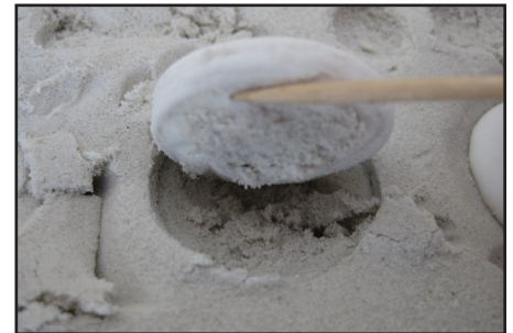
Once dry, use a toothpick to remove Casting Plaster button from Moon Sand.
