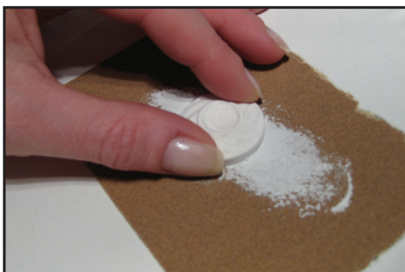
Clean Moon Sand off surface of Casting Plaster button using a toothpick and/or paintbrush. If necessary, sand bottom flat.
