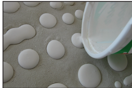
Mix Scene-A-Rama Casting Plaster in small plastic container as directed. Slowly pour into button impressions. Let dry for 30 minutes or until set.
